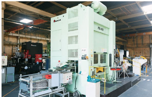
Presses with a pressure capacity of 400t (PDL) to handle high-tensile steel sheets
