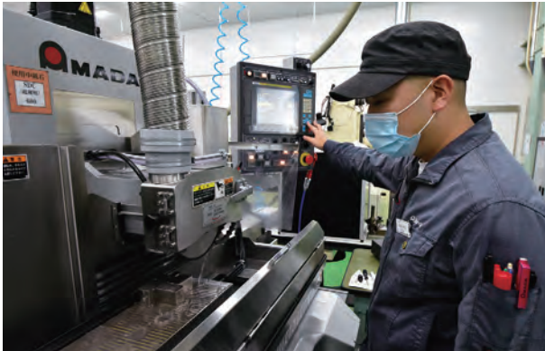
Picture of polishing of molding parts
